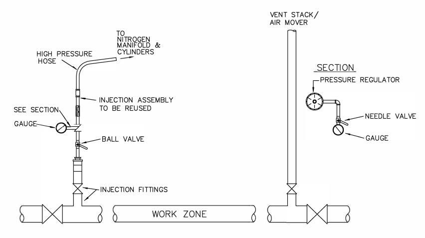
TYPICAL DETAIL FOR REPLACEMENT OF AIR WITH NATURAL GAS UTILIZING SLUG PURGE
