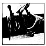
Tuck the gasket flap in place and mesh the lug fingers. Engage the center most bolt(s) in the drop-in lugs, and tighten finger tight.
