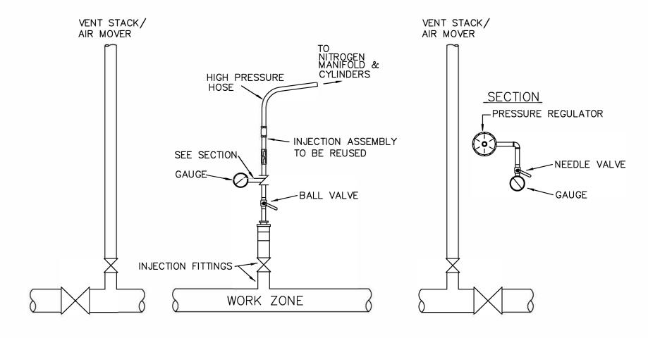
TYPICAL DETAIL FOR REPLACEMENT OF NATURAL GAS WITH AIR UTILIZING SLUG PURGE
