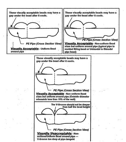
FIG. 4 Outside Diameter Butt Fusion Bead Guideline
