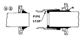
6. Stab the other pipe end into the middle ring until the end of middle ring meets the chalk mark. Pull out pipe ½" to allow for expansion. Slide gasket "M" into final position.
