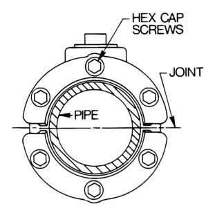
This is a preassembled sleeve ready for installation. DO NOT cut any gaskets, or remove any parts (except the side bolt hex nuts). Loosen the end capscrews 1 TURN only to remove the wooden blocks.
