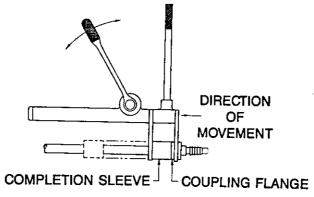
• REMOVE TOOL FROM PIPE AND REPEAT STEPS 1 THROUGH 5 ON SECOND SPIGOT OF THE COUPLING TO COMPLETE THE PIPE JOINT AS SHOWN.
