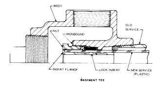
The style 88 Service Head Adaptors and Basement Tees for plastic pipe are recommended for a maximum operating pressure of 100 PSIG and a maximum temperature of 100 degrees F.
