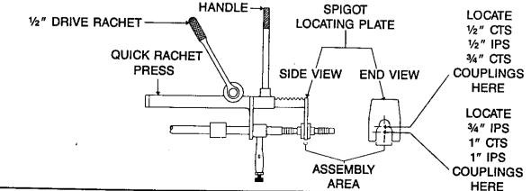
• OPERATE RACHET UNTIL PIPE COMPLETELY COVERS LAST SPIGOT BARB AS ILLUSTRATED IN STEP 2.
