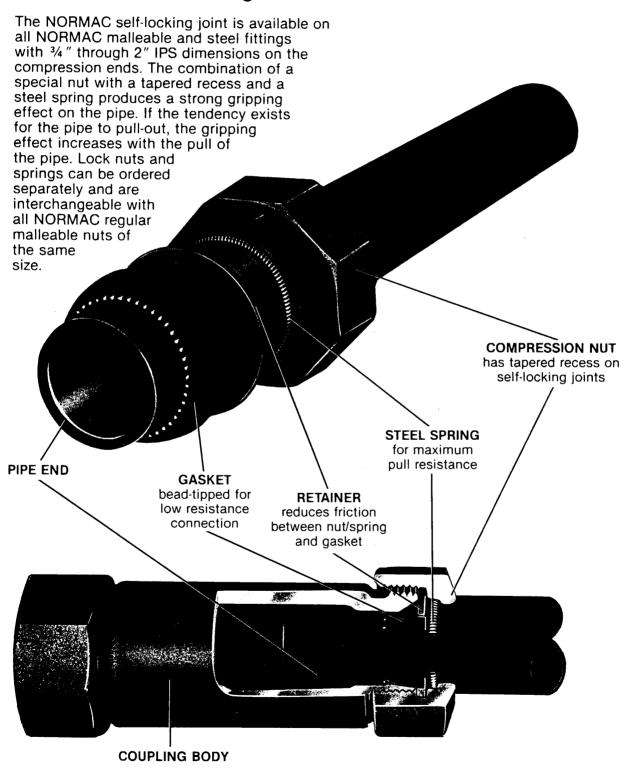
NOTE: This assembly shown is bead-tipped and self-locking. Plain gaskets have no beads, and fittings that are not self-locking use a regular compression nut and have no steel spring.
